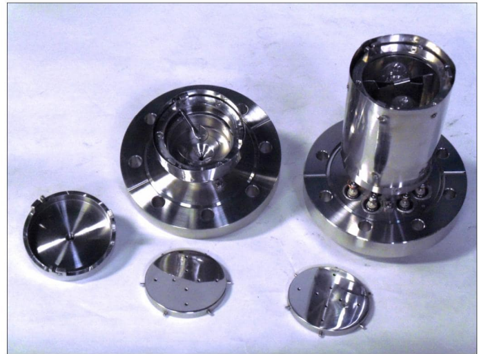
CF64 Supports for 2" RF sample holder and transfer pince
